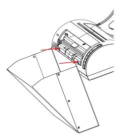
Finally, refit the tray in inclined position.
