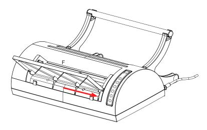
Lower the tray so that the tabs indicated in the figure slide into the slots, and move it with your hands following the slots (see figure).
